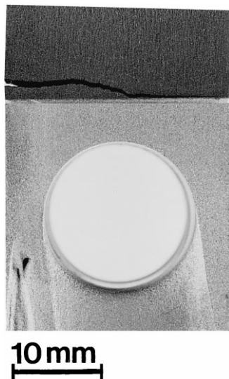
Fig. 8. Cross-section of the debonded divertor mock-up tested in the HHF cycling simulation (SiC 30-to-TZM module: 7 \text{ MW/m}^2 , 2 cycles).
